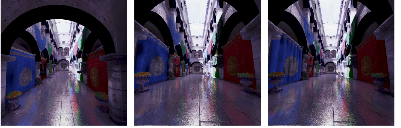
(a) Rendering for 128 voxel resolution (b) Rendering for 256 voxel resolution (c) Rendering for 384 voxel resolution
